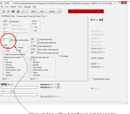
"1" revolution without ignition is not necessary. With "0", the engine starts more quickly
