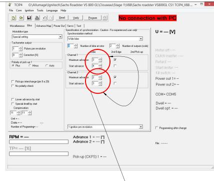
Sometimes, the wires of channels are inverted. So you must reverse the numbers of lobes in the software
